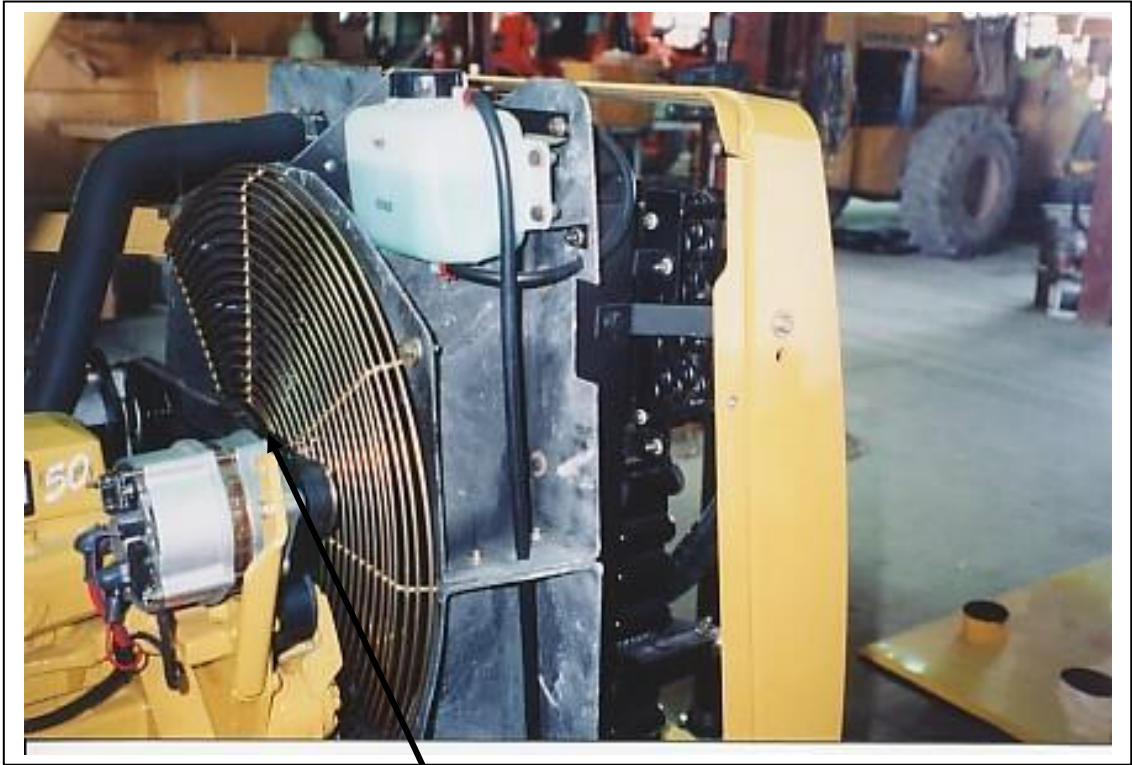
Aux. Pulley for the compressor
