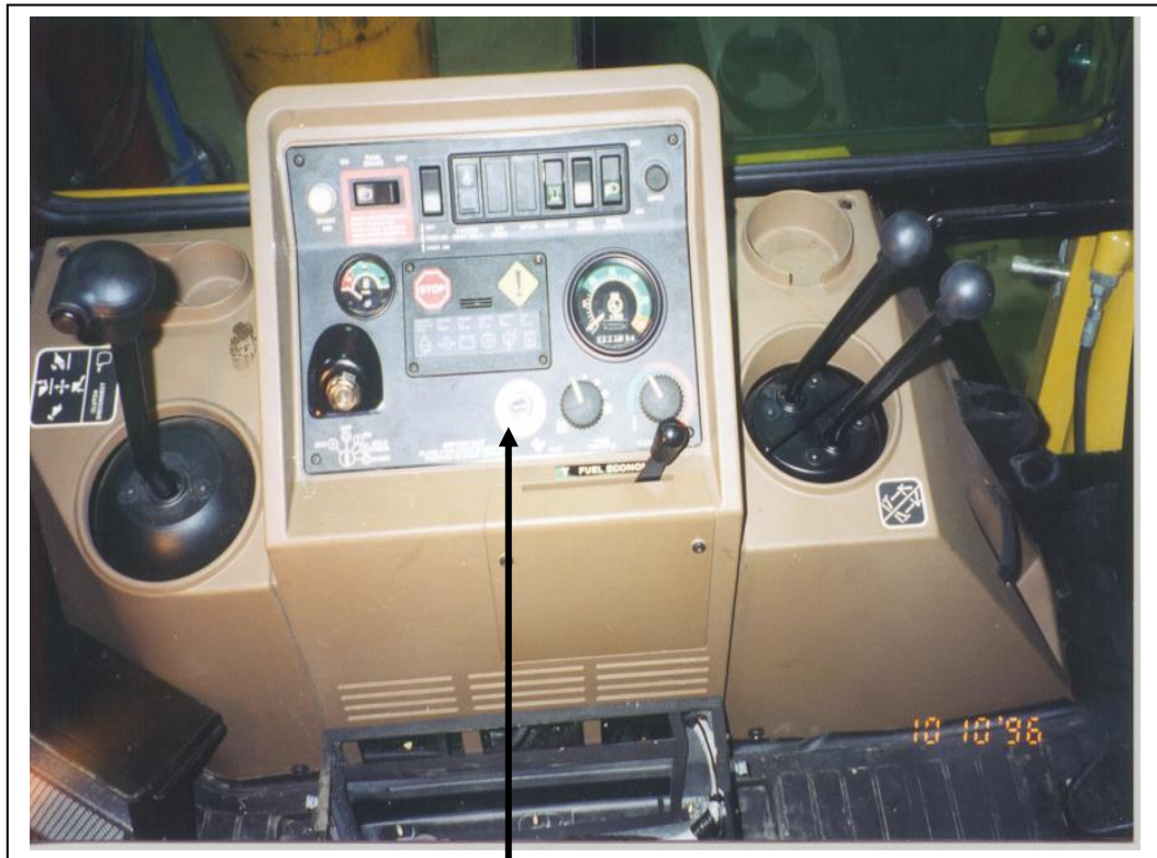
Thermostat installed in dash.
